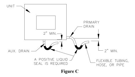
**NOTE:** Drain lines must be pitched no less than 1/4" per foot away from the air handler.
